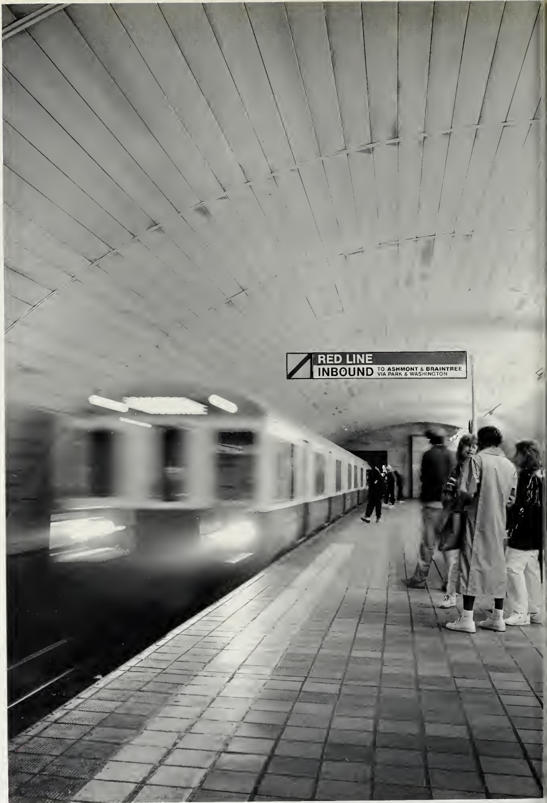
The new Red Line cars are made of stainless steel and are built in the United States. They are 100 feet long and 10 feet wide. They can carry up to 1,000 passengers. The new cars are expected to be in service by 2000.
